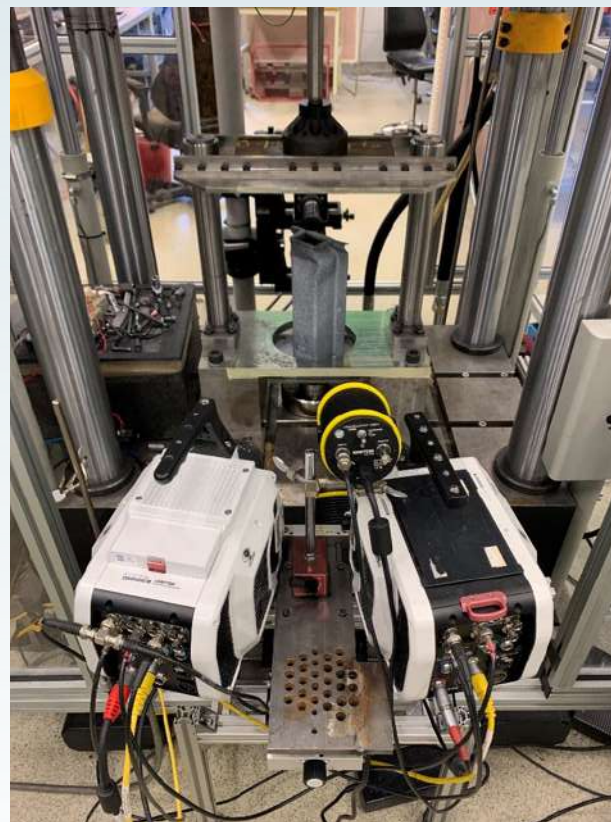
Two high-speed cameras - Vision Research Phantom v1610 and v2512 GOM – ARAMIS – DIC measurement system
