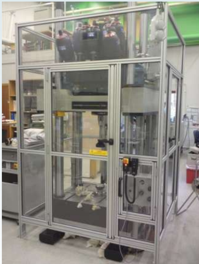
Instron VHS160/100-20, max ram speed 20 m/s
